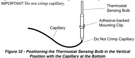
POSITIONING OF THERMOSTAT SENSING BULB For Masonry and **Factory-built Metal Fireplace**
